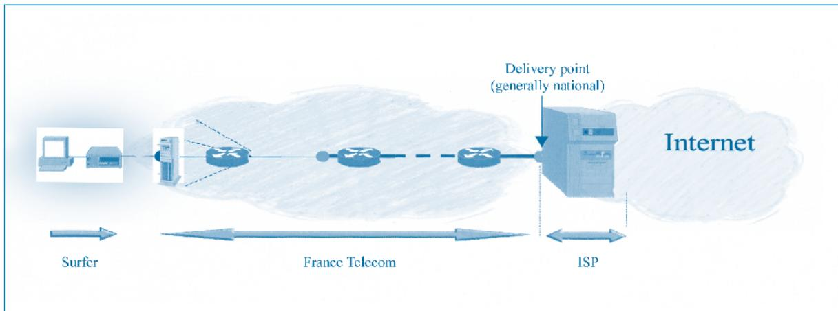
2) (Option 3) Operators buy a DSL traffic collection service on France Telecom's local loop and resell a global ADSL access and collection service to ISPs. ADSL subscriber traffic is delivered by France Telecom to a carrier at the regional level (40 delivery points). This carrier then extends collection to the ISPs' servers. ISPs are independent of France Telecom for part of collection allowing them to better distinguish their prices and quality of service (bandwidth per subscriber).
