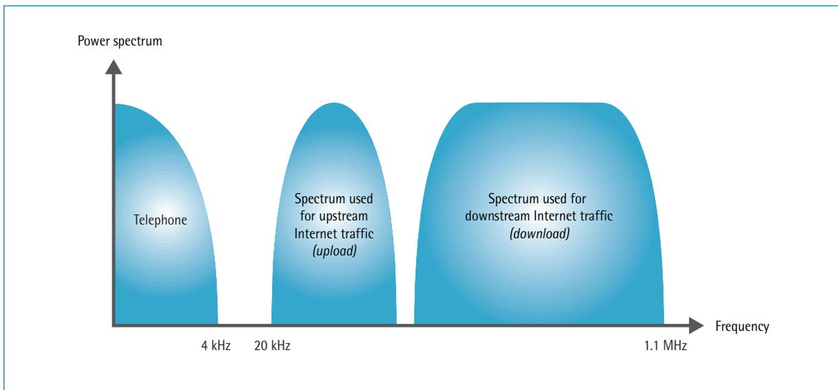
*Internet traffic is carried on the copper pair just like telephone traffic, from the user's computer to a distribution frame, the first element on the switched telephone network. At this point, it is separated from telephone traffic and routed to a separate IP network.*
