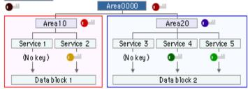
NFC applications are organized generically in the SIM card's memory. The security level of data access can be parameterized for each service.
